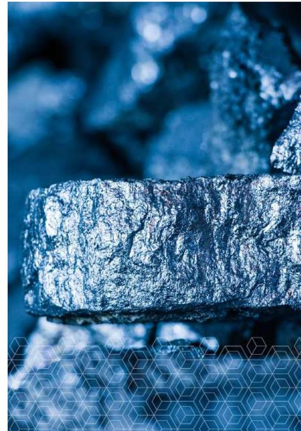
The main process:  $\text{SiO}_2 + \text{C} = \text{Si} + \text{CO}_2$
